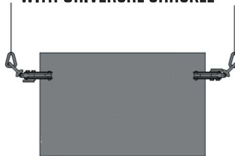
Designed to also lift material from the side
